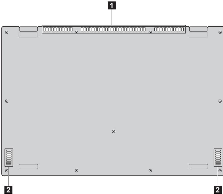
**1 Ventilation slots** Dissipate internal heat.
